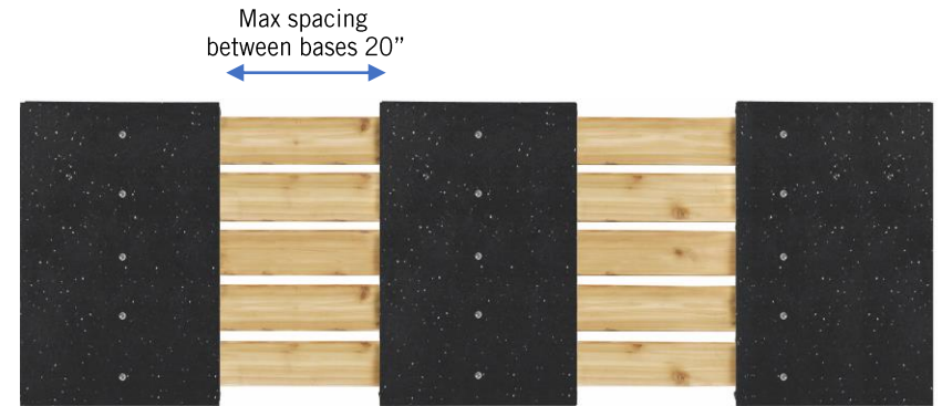
Fig 2. Starter panel, bottom view. Fasten base to 2x4' lumber, upside down, with 2" screws placed one screw per board, on center)
