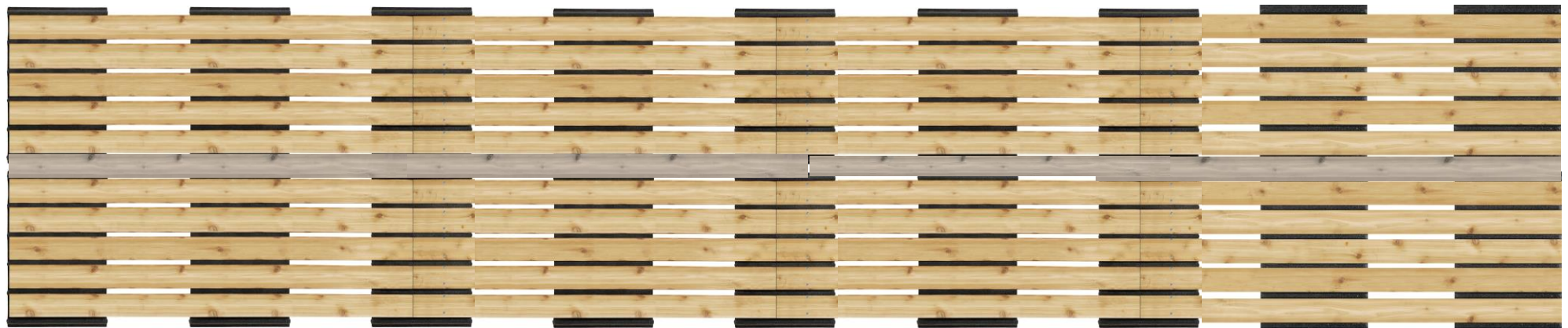
Fig 8. Add joiner boards along the entire length of the path, securing the joiner board by screwing into the top of the wood and down into the side supports of the base.
