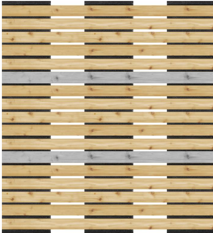
Fig 3. Align panels 4" apart and place a joiner board between the panels on the side supports of the SmartPath bases.
